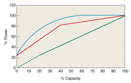
Single-Stage Lubricated Load/Unload (The graph represents one gallon of storage per cfm.)
