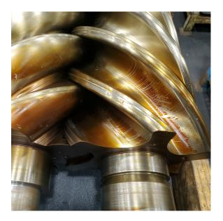
Varnish on an air compressor's rotors can occur when the wrong lubricant is used or if the lubricant isn't changed at regular intervals. Oil sampling can help identify when it is time to change out the lubricant.
