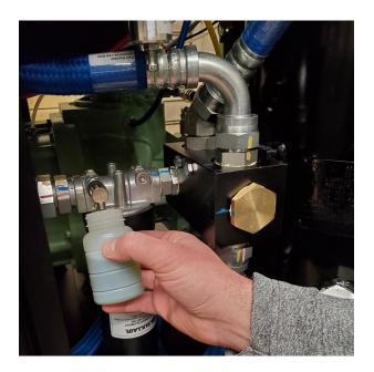
*Oil sampling provides a snapshot into the health of an air compressor. Regular sampling can help prevent costly downtime.*
