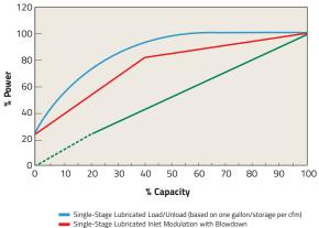
Single-Stage Lubricated Inlet Modulati
