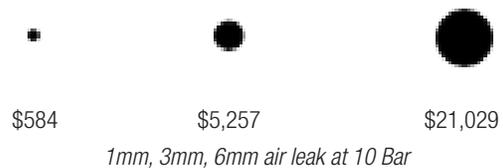
Air leaks can account for a big proportion of unplanned operational costs. An air leak from a 1mm orifice or hole can account to 0.38 kWh assuming 200C, 7 bar network
