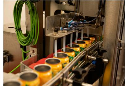
Compressed air is vital throughout Ghostfish Brewing Company's canning process—from affixing can tops, to blowing water off the top of the cans, to applying plastic can carriers. Additionally, compressed air is used in the keg washing process.
