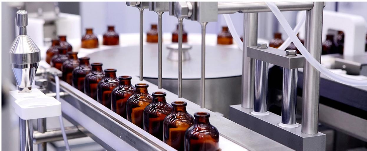
Compressed air is in a key component in many pharmaceutical manufacturing operations. Air power is used in processes such as tablet manufacturing, cleaning and drying, transporting products, packaging and more.<sup>1</sup>
