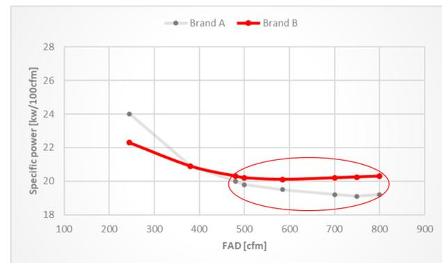
Sullair DSP VSD compressors are designed to operate in the blue circle, or what is known as the optimum efficiency range. Inside this blue zone, a VSD compressor runs at high efficiency and performance. Outside of this blue zone, the VSD compressor runs at low capacity and is inefficient with poor performance. This also comes along with some risks, including:
