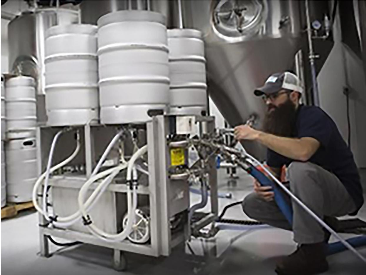
When speaking with a microbrewery, we learned about other usage of the compressed air. Many breweries use the compressed air for cleaning and canning applications. When washing kegs, breweries use compressed air to push cleaning agents through the keg washing process. In addition, it is used for keg purging after sterilization.
