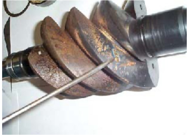
Signs of rotor coating degradation
