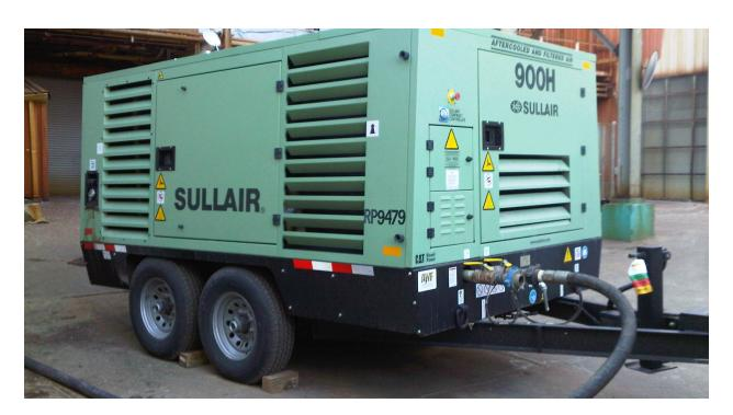
Compressed air is everywhere. Portable diesel air compressors bring compressed air wherever it is needed: plantside, roadside, refineryside and many other jobsites.
